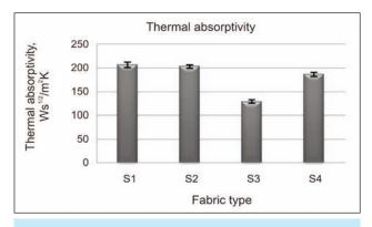
Fig. 8. Thermal absorptivity of the tested fabric sampless
