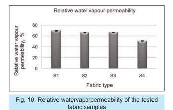
According to figure 10, nano-filament fabrics provided better water vapor permeability values because it has a larger surface area and nano-fiber structure which improve the transport system that pulls moisture away from the skin to the outer layer of the fabric. These fabrics are characterized by the small gaps between the fibers inside in the yarn. That's why the WPR of these fabrics is quite big as presented in table 4.
