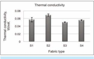
Fig. 7. Thermal conductivity of the tested fabric samples
