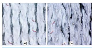
Fig. 3. Microscopic structure of Nano fibre polyester fabric S1 (a) and S2 (b)
