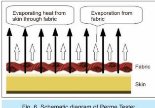
Fig. 6. Schematic diagram of Perme Tester
